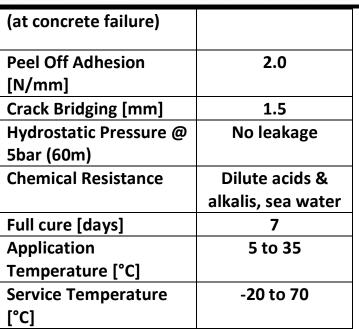
(The properties shown below were obtained under laboratory conditions). All values given are subject to 10% tolerance
