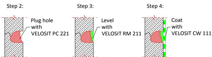
and push immediately into the prepared leakage. Hold for 1 to 2 minutes until the product has sufficiently hardened. Immediately shave the surface flush with the substrate. After a short waiting time
